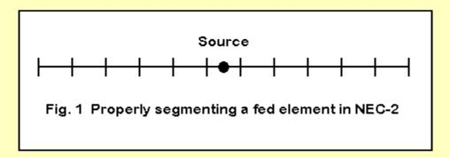
Segment length should be under 0.1 wavelength long, with 0.05 wavelength preferred (about 10-11 segments per half-wavelength). Segments shorter than 0.001 wavelength should also be avoided. For reference, the following table provides a ham band list of the maximum and minimum recommended segments lengths.
