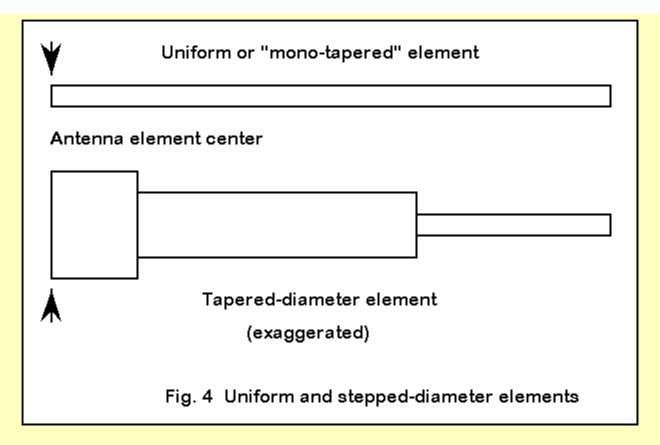
If an element is constructed on each side of center by, say, only 2 wires of different diameters and the junction of these wires is past the mid-point on each side, modeled results will be more accurate than with elements having multiple diameter steps closer to the center. Large steps in diameter also increase the accuracy problem.
