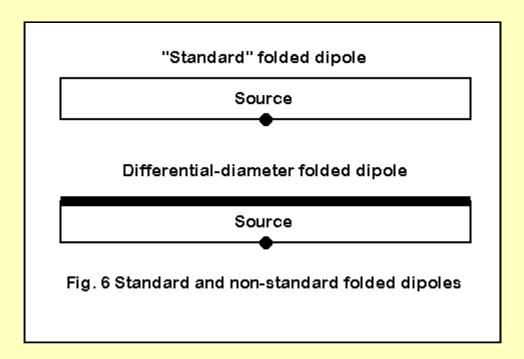
Folded dipoles using dissimilar diameter wires add another dimension to the NEC-2 limitations. Consider two folded dipoles, as shown in Figure 6. One consists of 2 parallel wires 0.5" in diameter spaced 0.25' apart and 16.1' long for 28.5 MHz. The other consists of one 0.5" diameter wire and
