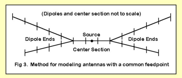
The simple work-around is also shown in Figure 3: adding a small common section of wire for the source and joining the diverging elements to the ends of this wire. Recommendations for these segments include a minimum length of 0.02 wavelength and 3 segments. Equally important, the adjoining segments of the diverging wires should be about the same length as those in the center section.
